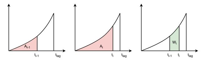
The weight array can be defined by giving the area below the lag function as a function of the time coordinate. The maximum lag  $t_{\text{lag}}$  must also be specified. The weights are then given by differences between the values of the area at consecutive lags. This approach is shown in the figure above, where the weight  $W_i$  is calculated as the difference between areas  $A_i$  and  $A_{i-1}$ .
