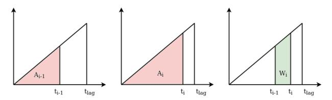
The half-triangular lag function grows linearly until  $t_{\text{lag}}$  and then drops to zero, as shown in the schematic. The slope  $\alpha$  is determined from the constraint that the total area of the triangle must be equal to 1.
