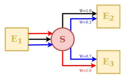
A Splitter is an element that receives the outputs of a single upstream element and distributes them to several downstream elements.
