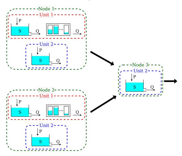
A catchment can be composed by several subcatchments (nodes) connected in a network. Each subcatchment receives its own inputs, but may share parameter values with other subcatchments with the same units.
