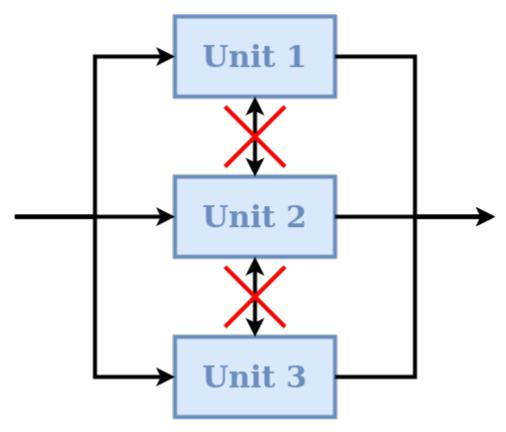
A node is a collection of multiple units assumed to operate in parallel. In the context of semi-distributed models, a node represents a single catchment and the units represent multiple landscape elements (areas) within the catchment. A node can be run either alone or as part of a bigger *Network*.
