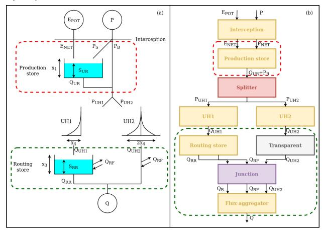
The potential evaporation and the precipitation are "filtered" by an interception element, that calculates the net fluxes
