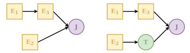
A transparent element is an element that returns, as output, the same fluxes that it receives as input. This element is needed to fill "gaps" in the structure defining a unit. See *Unit* for further details. An example is shown in the schematic above where the transparent element is used to make the two rows have the same number of elements.
