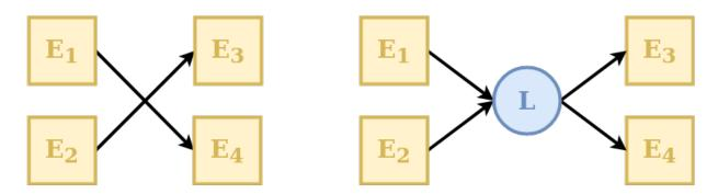
A Linker is an element that can be used to connect multiple elements upstream to multiple elements downstream without mixing fluxes.
