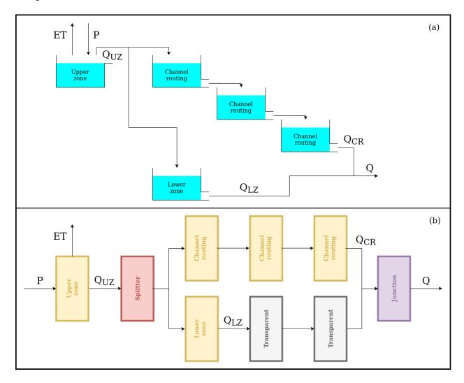
HYMOD comprises three groups of reservoirs intended to represent, respectively, the upper zone (soil dynamics), channel routing (surface runoff), and lower zone (subsurface flow).
