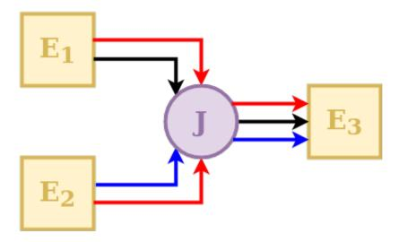
A Junction is an element that receives the outputs of several upstream elements and directs them into a single down-stream element.
