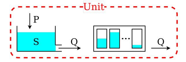
We now move to a more complex model structure, where multiple elements are connected in a unit. For simplicity, we limit the complexity to two elements; more complex configurations can be found in the *Application: implementation of existing conceptual models* page.
