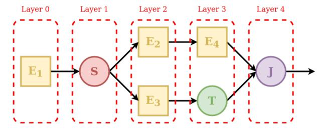
A unit is a collection of multiple connected elements. The unit can be used either alone, when intended to represent a lumped catchment model, or as part of a *Node*, to create a semi-distributed model.
