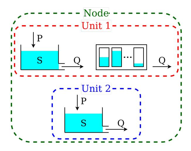
This model is intended to represent a spatially semi-distributed configuration. A node is used to represent a catchment with multiple areas that react differently to the same inputs. In this example, we represent 70% of the catchment using the structure described in *Lumped model structure with 2 elements*, and the remaining 30% using a single reservoir.
