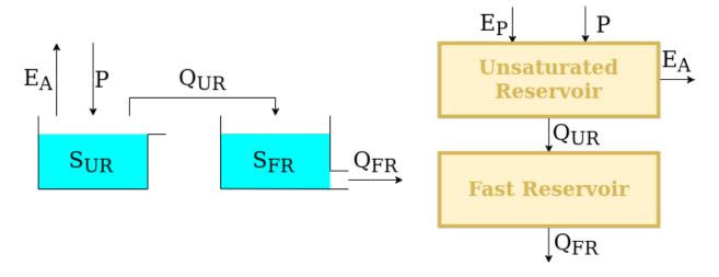
The upstream element, namely, the unsaturated reservoir (UR), is intended to represent runoff generation processes (e.g. separation between evaporation and runoff). It is controlled by the differential equation
