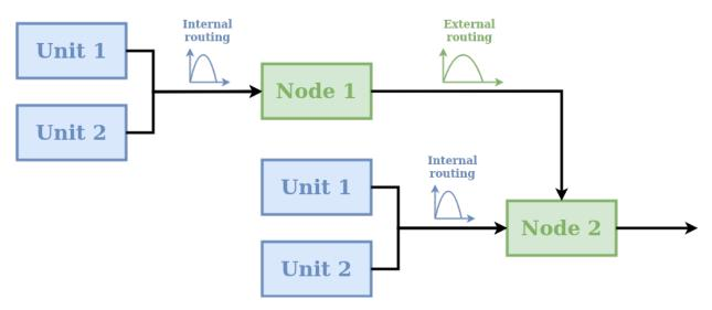
A node can include routing functions that delay the fluxes. As shown in the schematic, two types of routing are possible:
