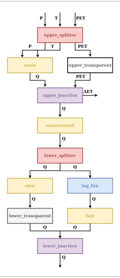
This model structure includes a snow model, and hence requires time series of temperature as an input in addition to precipitation and PET. Inputs are assigned to the element in the first layer of the unit and the model structure then propagates these inputs through all the elements until they reach the element (snow reservoir) where they are actually needed. Consequently, all the elements upstream of the snow reservoir have to be able to handle (i.e. to input and output) that input.
