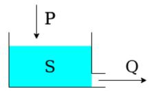
The single-element model is composed by a single reservoir governed by the differential equation
